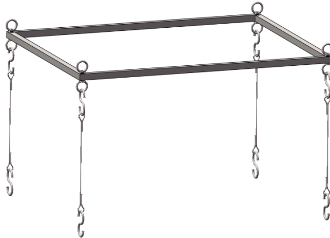
Figure 13: Lifting Tool for MYTEX U1L Modules
